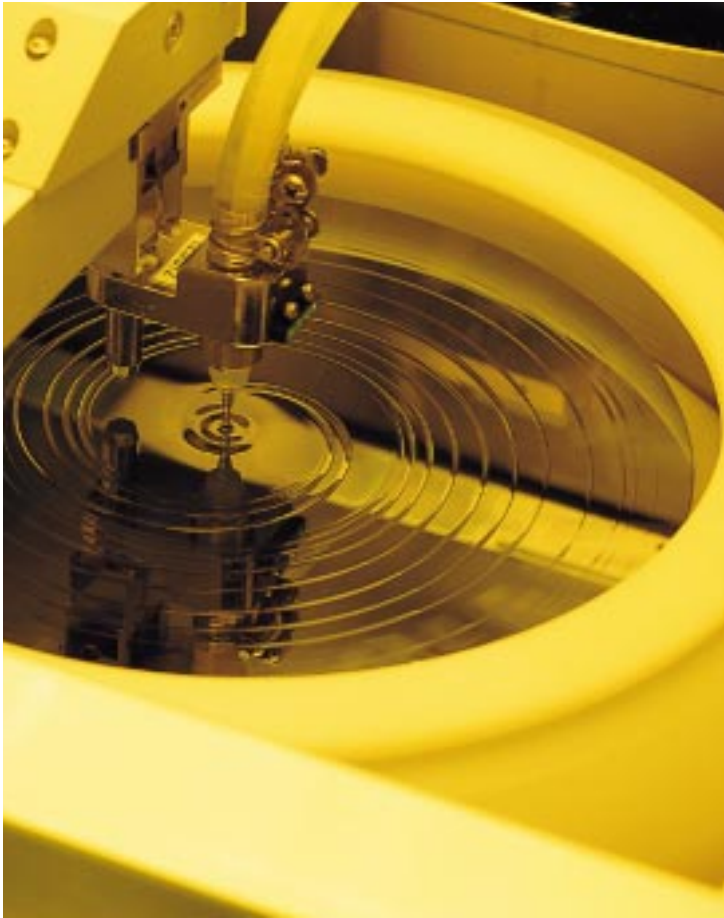
Photoresist in the photolithography process. Photolithography for semiconductors requires high resolution of photoresist chemicals.
