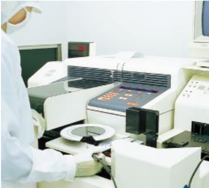
A Shin-Etsu technician manufactures epitaxial wafers by growing a microscopic layer of silicon on the surface of a silicon wafer.
