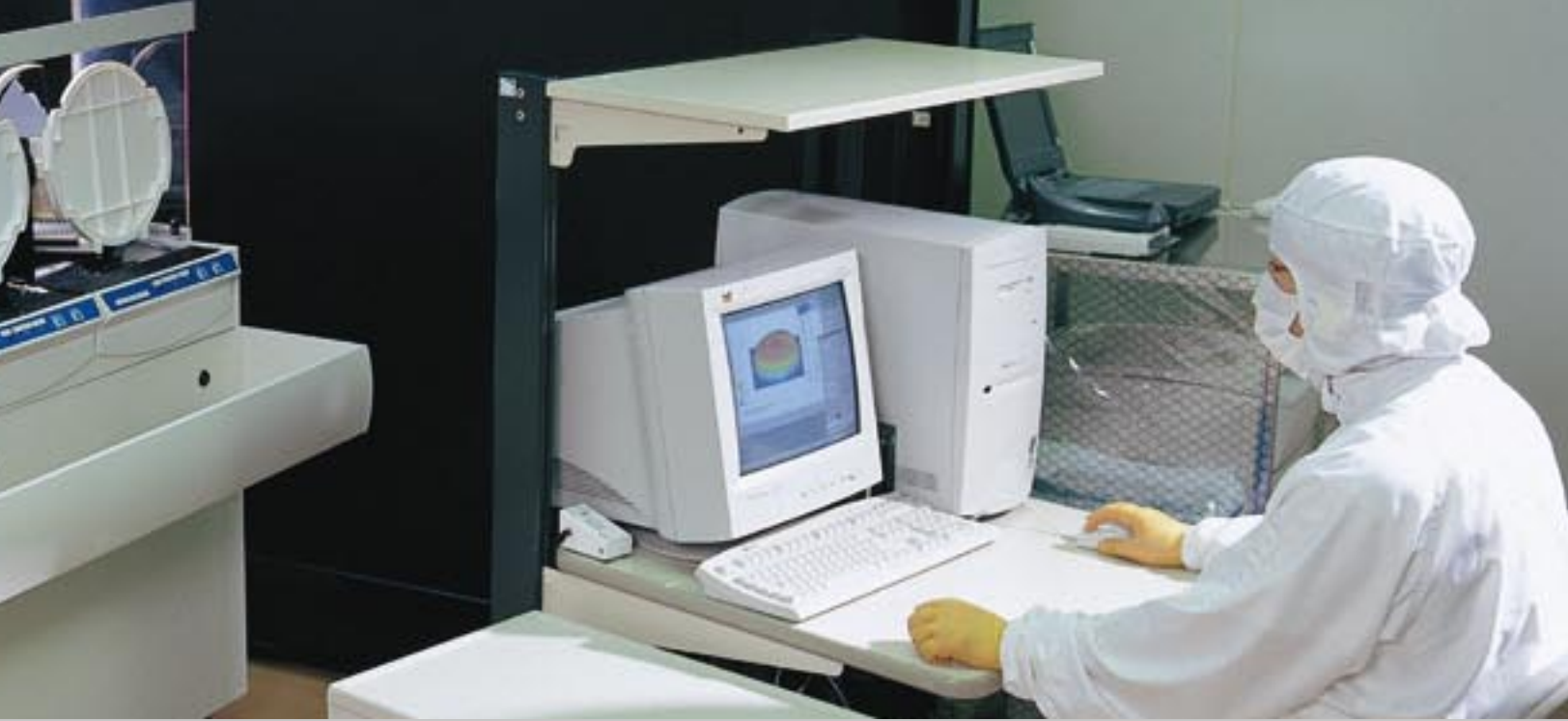
The production of 300mm-diameter silicon wafers demands the highest level of technology at every step through final testing. Shown here is the critical surface finish inspection.
