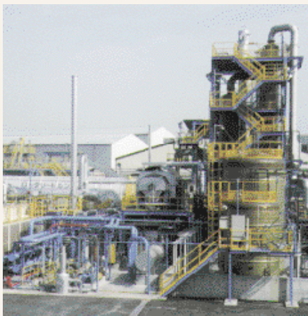
PVC used as a reductant in a shaft furnace: proof of the great contribution the recycling of waste PVC can make.
