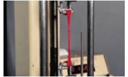
Testing the tensile strength of Silicone Rubber
