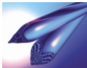
Optical-fiber preforms with diameters of 160mm and lengths of 1,500mm will eventually become roughly 2,000km of optical fiber.
