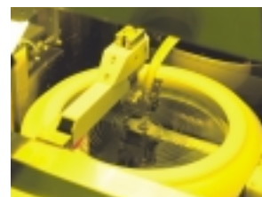
Photoresist spin-coated onto a wafer
