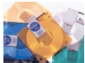
Rare earths also have applications as recording materials in MO, MD, and other magneto-optical disks.
