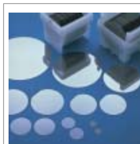
Silicon wafers boast a degree of evenness to within 0.1 micrometer.
