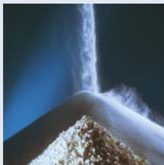
Shown here are white powder-form PVC polymer and pellet-form compounds
