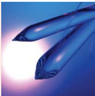
Optical-fiber preforms with diameters of 160mm and lengths of 1,500mm will eventually become roughly 2,000km of optical fiber
