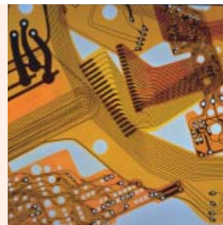
Flexible copper-clad laminates essential for flexible printed circuit boards (FPCs)
