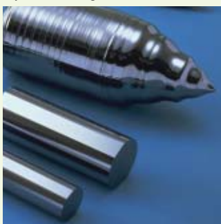
Examples of wide-rimmed single crystal silicon ingots
