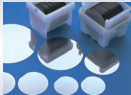
Silicon wafers boast a degree of evenness to within 100 nanometers.
