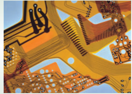
Flexible copper-clad laminates essential for flexible printed circuit (FPC) boards
